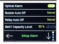
The visual and audible alarm can always be acknowledged in advance by touching the screen, or can automatically switch off after a definable time.
