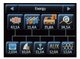
By touching the source symbols, the current display can be switched to show the amperehours supplied or consumed since the last counter reset. The display changes back to the current display automatically after 1 minute.
