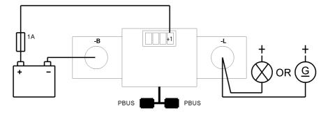
At the shunt SHL the 4 pin. connector is connected as follows:
