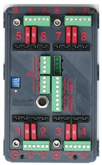
The wire cross-section of the power supply lines (+ and -) must correspond to the sum of the 4 output fuses. 4 x 10 A correspond to a total current of 40 A and therefore the supply line must have a minimum cross-section of 6 mm<sup>2</sup>. This supply line must be fused at the battery according to the line cross-section.
