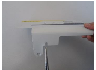
Break out the metal tongue with a pair of flat-nose pliers
