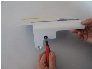
Inserting the rubber cable grommet
