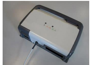
Insert the cover and the cable
