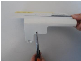
Break out the metal tongue with a pair of flat-nose pliers
