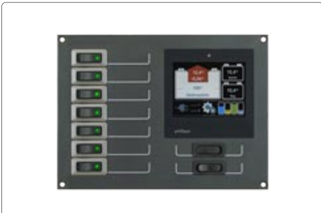
STV 237 (BTM) Order-No.: 0 2000 2370 STV 247 (PSM2) Order-No.: 0 2000 2470 7 power circuits with thermal circuit breakers 10 A, monitor BTM or PSM2 and 2 control switches for individual use. Shunt SHE (BTM) or P-BUS components have to be ordered separately! Dimensions W 210 x H 157,5 x D 70 mm Suitable terminal blocks type RKL 10
