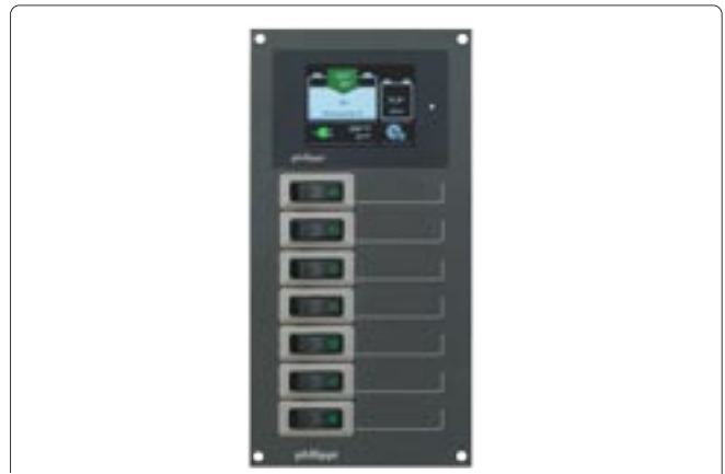
STV 216 (TCS) Order-No.: 0 2000 2160 STV 218 (BLS-Set) Order-No.: 0 2000 2180 7 power circuits with thermal circuit breakers 10 A, monitor TCS or BLS-Set. The shunt SHE 300 is included in the scope of delivery of the STV 218. Further information about the monitors on page 45ff. Dimensions W 105 x H 210 x D 70 mm Suitable terminal blocks type RKL 10
