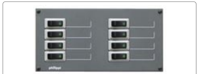
STV 208 Order-No.: 0 2000 2080 8 power circuits with thermal circuit breakers 10 A Dimensions W 210 x H 105 x D 70 mm Suitable terminal blocks type RKL 10
