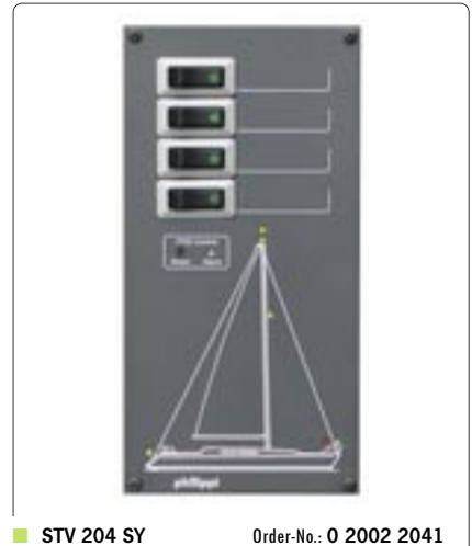
STV 204 SY Order-No.: 0 2002 2041 4 power circuits with thermal circuit breakers 10A, display sailing yacht incl. electronic navigation lights monitor POS 6 with alarm, for use with LED -lanterns or normal bulbs, for 12V and 24V Dimensions W 105 x H 210 x D 70 mm
