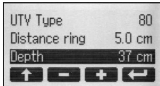
If the tank depth plus the distance ring is equal or less than 40 cm you need an UTV 40; greater than 40 cm an UTV 80. The TCM4 shows the type of UTV- sensor required automatically.
