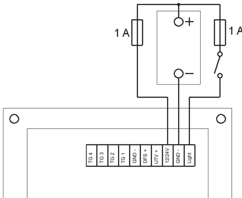
Connection of ultrasonic sensor UTV or over active sensors:
