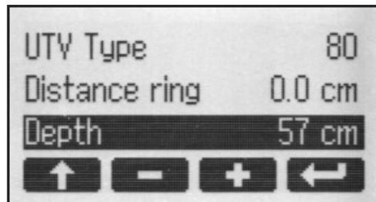
To balance the off zone of the ultrasonic sensor (the range which is not measurable between sensor and liquid surface - 50 mm) you can use a distance ring UTS 25 or UTS 50.
