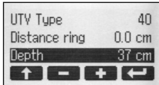
Is the depth of the tank greater than 40 cm, you have to use an UTV80. The TCM4 is showing that automatically:
