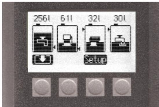
If an alarm threshold for a tank is set up, this threshold is shown by a little triangle on the side of the bar. So you have a quick overview if the tank level is inside of the correct range.
