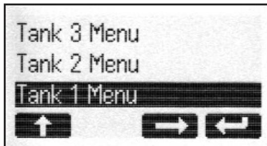
in the tank menu you can adjust the tank type (e.g. water, fuel, waste and the type of the sensor), the capacity, the compensation-value (adjustment of the tank-geometry), the alarm-threshold and duration. Also you have the possibility to preset the ohm-values for 0%, 50% and 100% if your sensor has another range of resistance than 5 - 180 or 240 - 33 ohm (tank type 25 -29).
